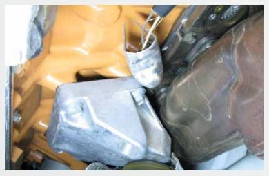
Repeat same steps as driver's side but you will also have to remove dip-stick and remove alternator brace bracket. (Note: you will be re-using dipstick bolt and nut for install).
