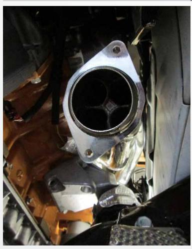
Install BBK headers with supplied gaskets and hardware making to use dipstick bolt and nut. Re-attach alternator brace and install motor mount. Then install factory head pipes. Remove factory O² sensors from manifolds and install them into BBK headers using anti seize. Install factory plastic shields and start vehicle checking for any leaks. Re-torque all header fasteners the following day after a couple of heat cycles.
