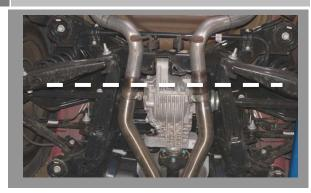
Cut the stock exhaust pipes 1-1/2" forward of where the rear end cover bolts to the third member. Use a sawz-all or air powered cut off wheel to cut the pipes.
