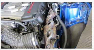
Remove the (5) bolts that secure the stock manifold to the cylinder head and remove the exhaust manifold and gasket from the vehicle.
