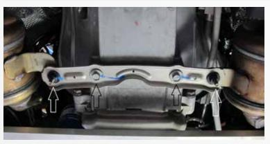
Loosen the (2) 13mm bolts and the (2) 13mm nuts on the cross brace. NOTE you do not need to remove it completely.
