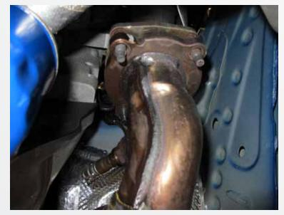
Remove the (4) 15mm nuts on the passenger side and driver side that secure the catted down pipe to the exhaust manifold.
