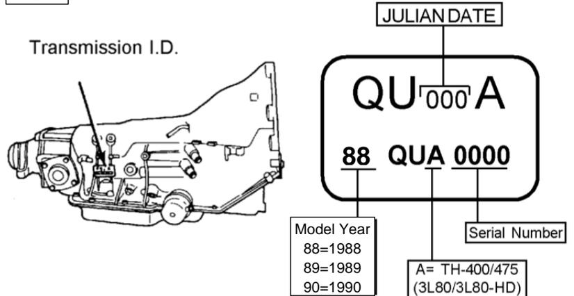
If the I.D. tag is unreadable or missing you will have to remove the oil pan and valve body from the transmission to determine if your transmission has an early or late style case (See Fig. 2). The manufacturing date check applies only to 1988 transmissions, this kit will work correctly in all subsequent application years specified in the heading of these instructions.
