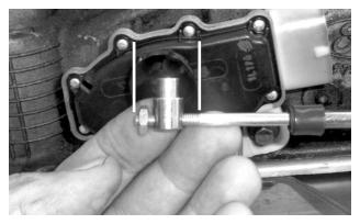
**22. Thread the swivel onto the cable** to about the middle of the threaded section, then reinstall (but do not yet tighten) the jam nut.
