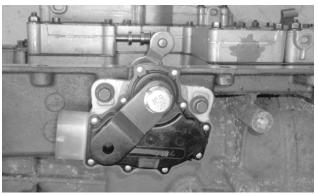
14. Install the selector lever on the shaft, using the supplied M10-1.5 × 20 bolt and M10 washer.
