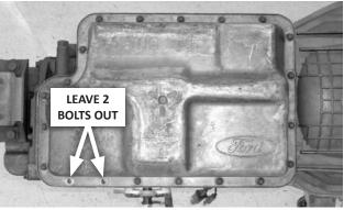
**17. Install the pan and new gasket** using 12 of the 14 the original bolts. (Do not tighten yet.) Leave out the 2 rearmost bolts on the driver-side flange for the cable bracket.
