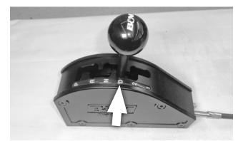
A. With the selector lever still in OD (from Step 20) and the shifter in DRIVE (or 3), adjust the cable bracket nuts (and swivel, if necessary) until the swivel slips freely in and out of the selector lever hole.
