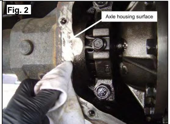
9. Verify what size cover bolts are used on your axle housing. These axle housings came with 3/8"-16 bolts or M8x1.25 bolts. Both size bolts are included in this kit.
