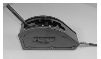
**10.** Ensure there is no debris in the shifter mechanism, then reinstall the assembled gate plate and side covers on the shifter base, using 3 screws along each side.
