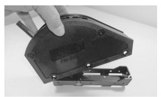
2. Disassemble the shifter: Remove the knob and jam nut from the shift lever. Remove the 3 countersunk screws from the bottom of each side of the shifter. Then remove the assembled gate plate and side cover from the shifter base.
