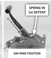
CAUTION: The shifter has two PARK positions — the first (lever full-forward) is for GM transmissions; and the second (one position back) is for Chryslers and Fords. To avoid stretching the shifter cable when shifting into PARK, NEVER force the shifter past the second (rear) PARK position (which corresponds to your transmission selector lever's PARK detent).
