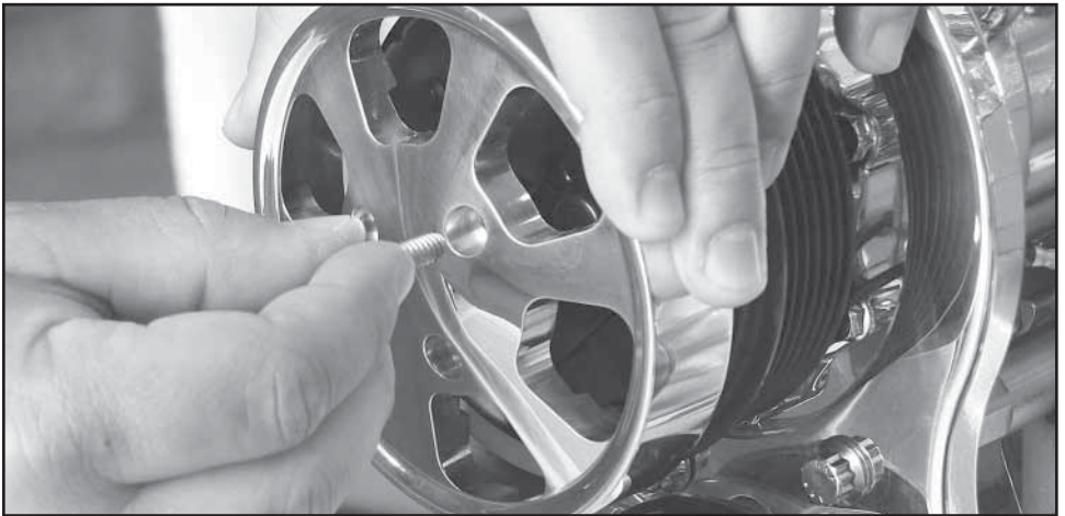
Figure 13: Install SD-7 Compressor Clutch Cover
