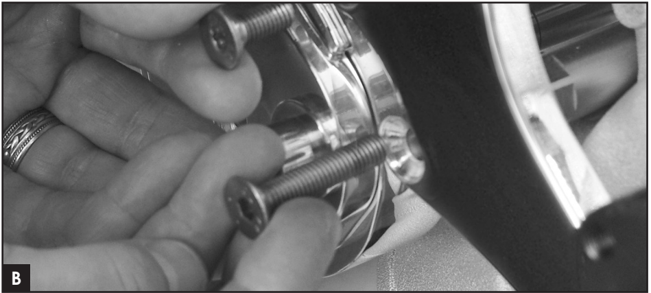
Figure 7: Attaching Bridge Bracket
