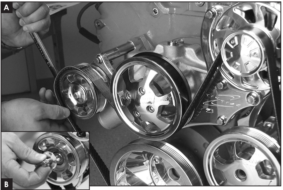
Figure 11: Install Serpentine Belt & Tensioner Pulley
