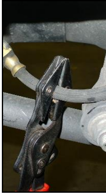
Figure 1: Vise grips applied to OE brake hose
