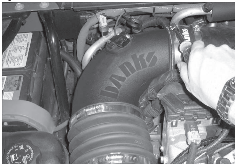
Figure 7- Secure Banks Intake Tube
