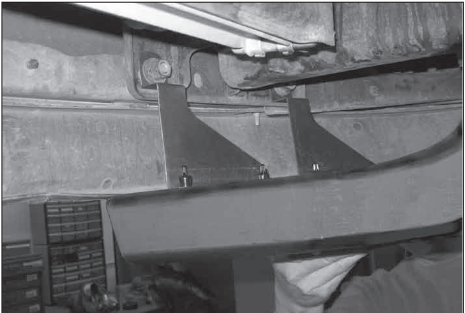
Figure 6 Install Super-Scoop support brackets over factory bolts
