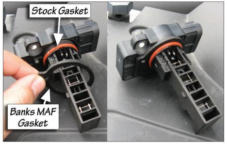
Figure 5- Remove Stock Air Filter Minder & Air Filter Minder Gasket
