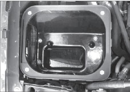
Figure 3-Position Cut-out to Face Passenger Side Fender
