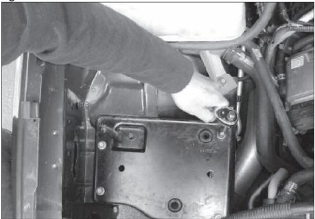
**7.** Locate your Banks Ram-Air filter housing from your kit. Align the Banks Ram-Air filter housing to fit parallel to fender edge. Install and tighten the previously removed bolts to secure the Banks Ram-Air filter housing.
