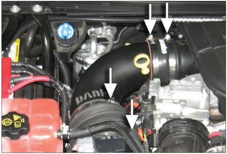
**18.** Locate the Banks turbo intake hose, tube, and hose clamps from your Banks Ram-Air kit. Loosely assemble the Banks intake hose to the Banks intake tube with the supplied hose clamps. Attach the turbo intake hose to the turbo intake tube. Leave the hose clamps loose.
