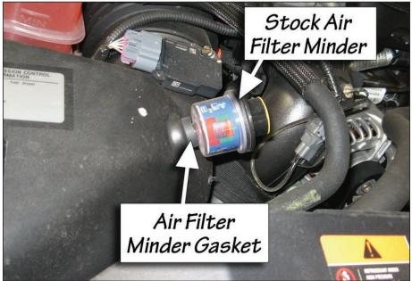
**11.** From the stock air box, remove the stock air filter Minder. Make sure to remove the stock air filter Minder's rubber grommet as well. See **Figure 5**.
