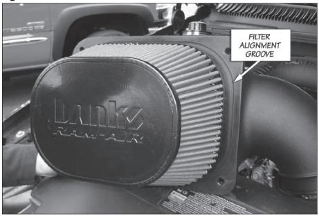
Figure 6- Align Locater Groove to the Banks Ram-Air Filter
