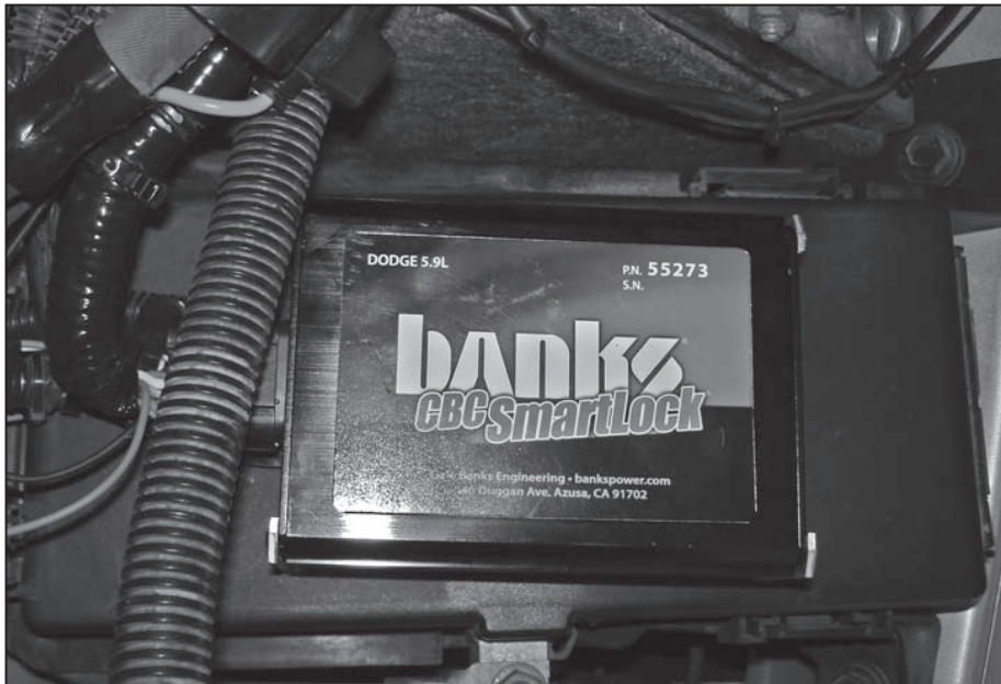
Figure 32 All Models CBC Smartlock Mounting Location
