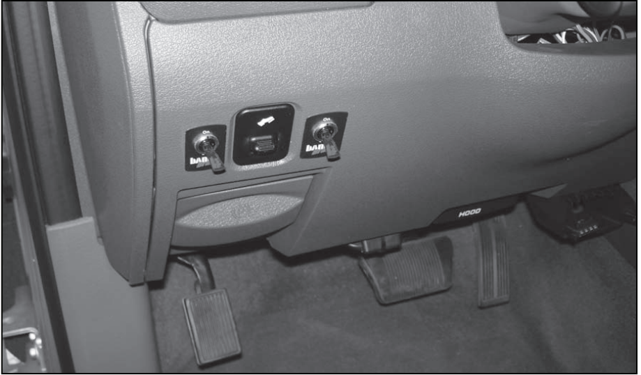
Figure 45 2006 Models Power Adjustable Pedal Switch Location
