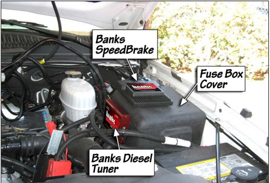
Figure 6 Placement of Banks Tuner on side of the Fuse Box.
