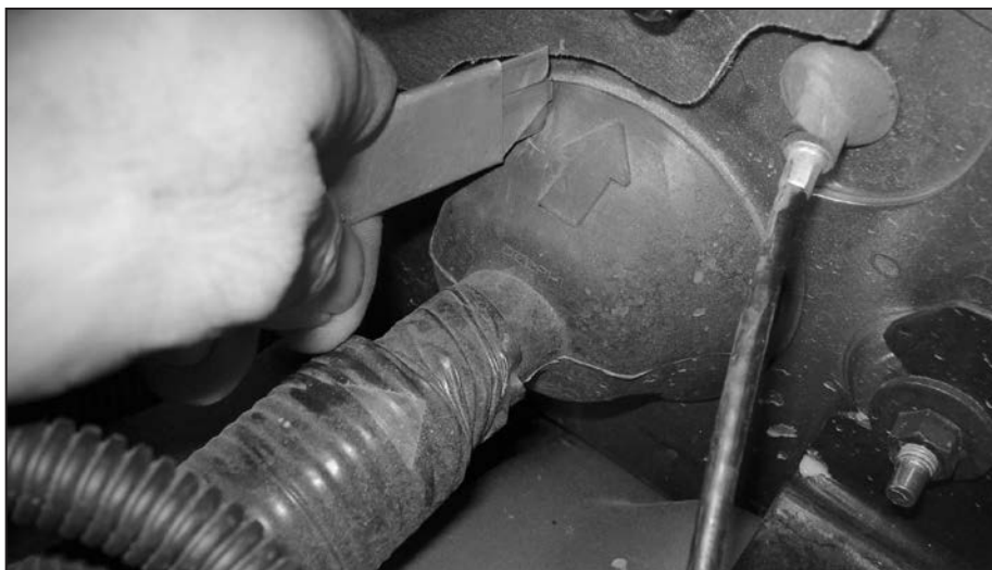
Figure 4 Driver Side Firewall, Rubber Grommet
