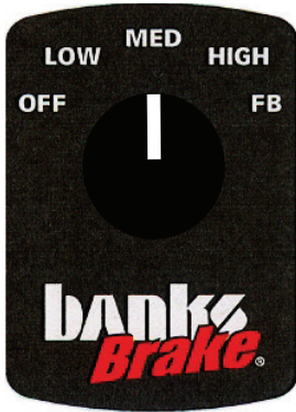
Figure 20: Banks Brake Selector Switch Guide
