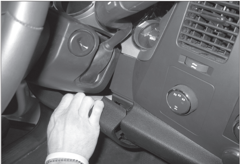
Figure 8 Removal of Knee Bolster
