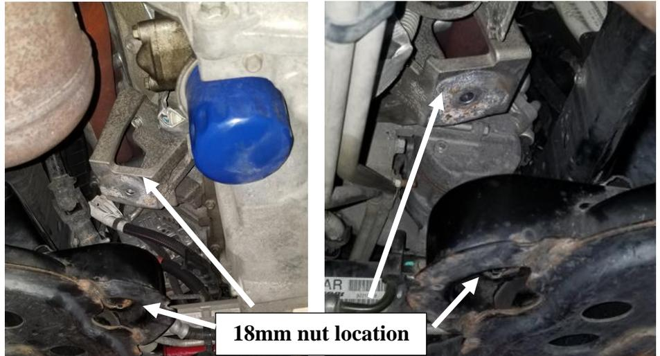
**NOTE: these motor mounts have two (2) ¼" THICK SPACERS ON each side. They allow you to lower the motor a total of ½" per side given proper oil pan/ swaybar/ steering rack clearance. Ensure clearance around motor before lowering motor from stock height.**
