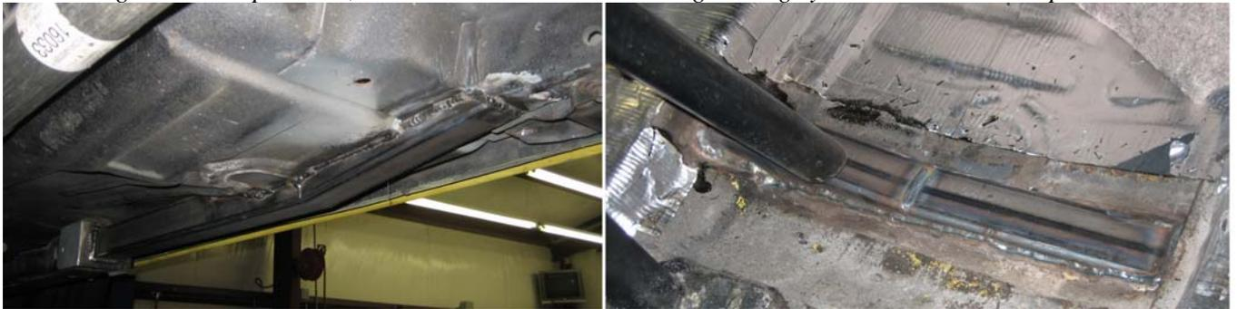
15. Lift the rear of the subframe connector up until it lines up with this bolt hole as shown in Image 3 below.
