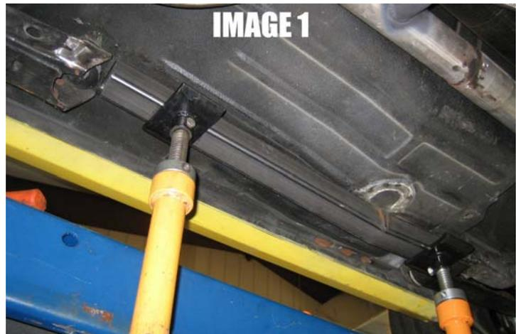
*NOTE: do not cut the entire length of the foot well. Stop the cuts at the body seams as shown in Image 2 below. The rear body seam is only visible from underneath the car while the front body seam is only visible from inside the car.*
