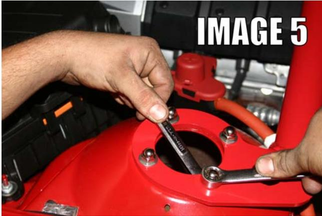
7. Lower vehicle, allowing the struts to return to their original position. It may require the help of another person to guide the strut mount up into the strut tower while the car is being lowered.
