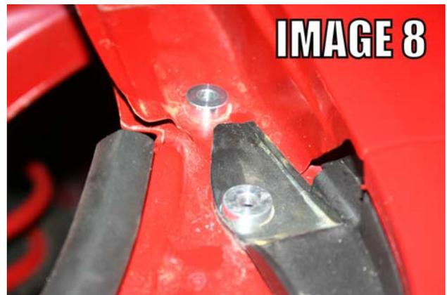
9. Install the provided billet strut retainer and the new provided 14mm jam-nut.
