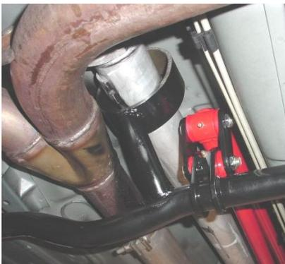
**OPTIONAL WELD-IN DRIVESHAFT LOOP INSTALLATION:** Remove one end of the driveshaft and slide the driveshaft loop over it. Reinstall driveshaft. Position the loop 6 inches from the front u-joint. Mock it up so that there is sufficient clearance to allow the driveshaft to go up and down 1.5". Using the provided length of tubing, cut and weld the ends to allow mounting the loop to the crossbrace. Double check the clearances and weld into place.
