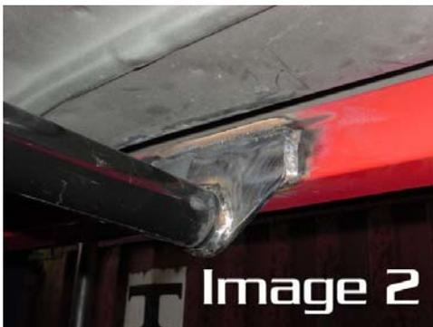
6. Reattach the pivot plates, attaching the crossbrace to the torque arm and tighten the bolts.
