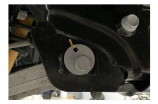
10. Use an 18mm socket to remove the sway bar end links.
