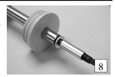
This process is not normally needed for the Belltech 2" drop but is recommended when lowering more than 2". This process will allow for additional adjustment to obtain factory spec alignment. If lowering vehicle less than 2", please skip to step 7.
