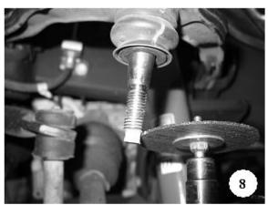
ball joints and loosely thread the nuts in place. It is helpful to use a jack or lifting device to raise the lower control arm while re-attaching the spindle ball joints. Be very cautious while lifting the lower control arm because it is under extreme load. Make sure the lifting device base is stable and the portion connected to the lower control isn't able to slip out.
