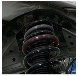
13. Remove the strut from the vehicle.
