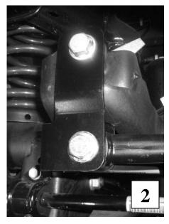
3h) Check all of the hardware and re-torque at intervals for the first 10, 100, and 1000 miles.
