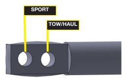
16. Attach the end links onto the Belltech bar using the original 18mm nuts. Torque to 16 ft lbs. once the vehicle is back on the ground.
