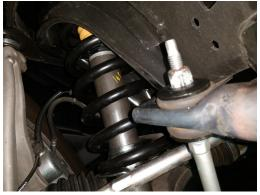
10. Remove the 15mm bolts holding the OE sway bar bushings in place. Remove the sway bar from the vehicle.
