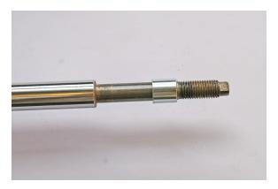
3. Install first washer below the bushing and bottom pin bushing; with selected notch facing up (see Pin Bushing section). When the shock is installed on vehicle, place the top pin bushing with selected notch facing down and the second washer above the bushing.
