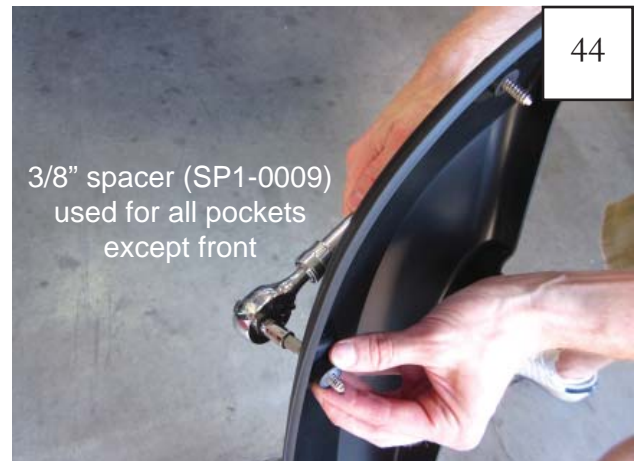
44 For all remaining pockets, install a #45 Torx screw (SW1-0045) through pocket hole and secure with rubber spacer ( SP1-0009 ) using supplied #45 Torx bit (SW1-0052). Drive screw into spacer until tight. Repeat for all remaining pockets.
