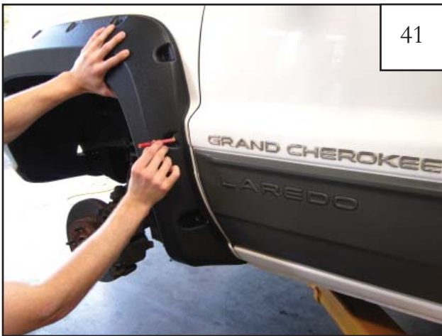
41 Hold flare in place on vehicle, mark hole locations on fender through holes drilled in pockets of flare.
