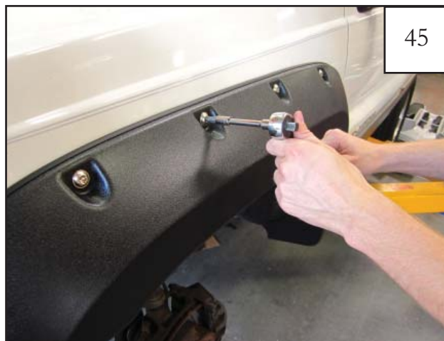
45 Hold flare in place on fender. Using the provided torx bit driver and ratchet with 3" extension, start each screw into drilled holes.
