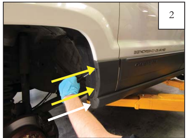
Using a #2 Phillips Screwdriver, remove factory screws from upper side cladding (2 places). For models with rocker panels installed, remove screw from end of rocker panel (1 place).
