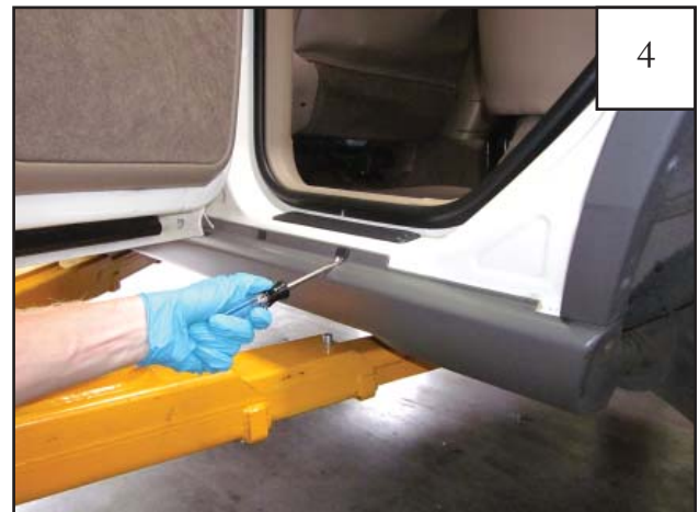
(Note: For models with Rocker Panels installed) Open front and rear doors. Using a pry tool, remove retainers along top of rocker panel.
