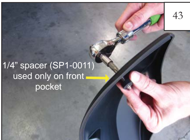
43 Install a Torx screw (SW1-0045) through FRONT pocket hole of flare and secure with rubber spacer ( SP1-0011 ) using supplied #45 Torx bit (SW1-0052). The torx bit fits into a 5/16" socket. Use with a 3-6" extension for drill or air ratchet. Drive screw into spacer until tight.
