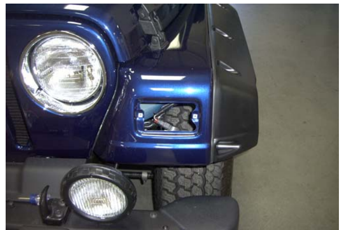
Photo #1 – Front Marker Light Cover Removed
