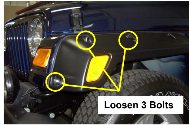
Photo #2 – Loosen Bolts (Do NOT Remove)
