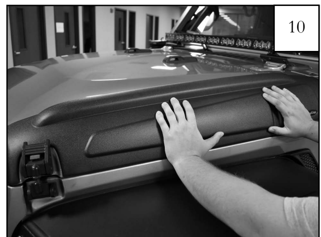
Apply FIRM pressure to all mounting locations to affix Trail Armor to vehicle.
