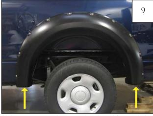
Using a 10mm socket wrench, reinstall factory bolts.
