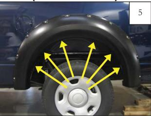
Hold flare to vehicle and mark the location with a grease pencil of the six holes in the flare.
