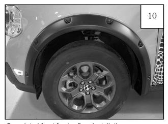
Completed front fender flare installation.
