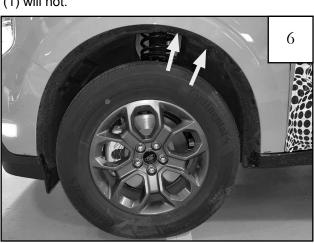
Remove and retain (2) additional factory fasteners.
