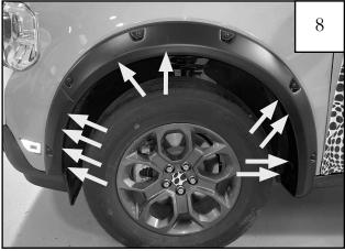
Position fender flare back in place on wheel opening and align with holes. Reinstall (10) previously removed factory screws.
