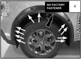
Hold front flare up to vehicle wheel opening. Use a grease pencil to mark (11) locations where holes in fender flare align with the wheel opening. NOTE: (10) locations will align with factory fasteners, and (1) will not.
