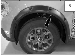
Install (1) SW1-0058 screw in the remaining hole to attach the fender flare to the bracket installed in **Step 7.**
