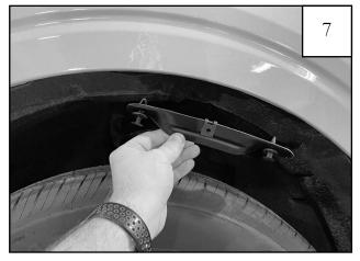
Install (1) front inner bracket, reusing factory fasteners removed in **Step 6**. *NOTE:* Both inner brackets are universal.
