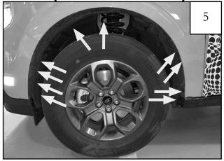
Set fender flare aside. Remove (10) factory fasteners from marked locations. Retain fasteners for reinstallation.
