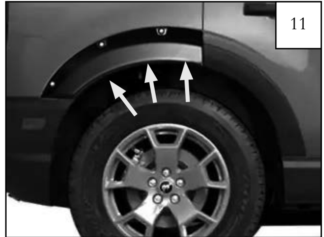
Position flare on fender. Note the (3) slotted fastener locations in the flare.
