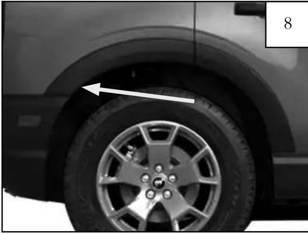
Remove (1) factory installed plastic fastener from the rear of the wheel opening to expose hole.
