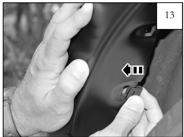
Press U-clip (122411) in place so that it encompasses both edge of fender flare and edge of factory fender trim, making sure that the retention tang of the U-Clip engages in the slot. Repeat for remaining slots.
