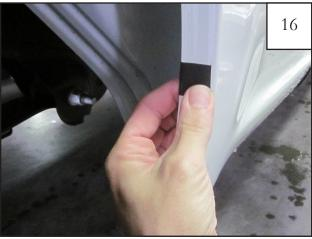
Wrap a Mylar Tab (MT1-0014) around the wheel well sheet metal, centered over each of the three marks made in Step 15.
