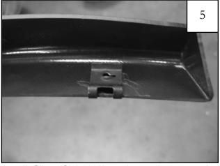
Install Clips (CL1-0022) on inner piece over the holes. (2 Locations)
