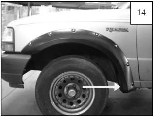
Reinstall factory screw saved from Step 8.
