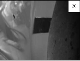
Install a Tab (MT1-0002) centered over each of the four holes marked in Step 19. Edge of Tab should be even with edge of sheet metal.
