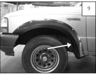
Hold flare to vehicle and mark second rearmost hole location with grease pencil.
