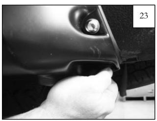
Start Fender Brace Nut removed in Step 17 on fender brace bolt.
