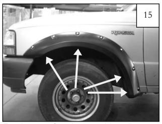
Ensuring proper flare placement, tighten all screws.
