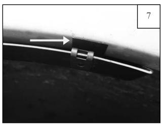
Install Tab (MT1-0002) on sheet metal between inner piece and wheel well at two inner piece Clip (CL1-0022) locations. Tighten factory screws.
