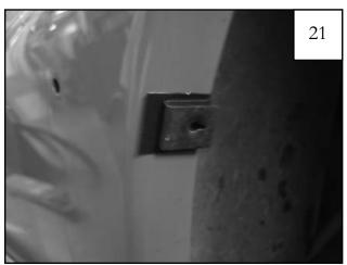
Install an Clip (CL1-0005) over each of the Tabs installed in Step 20.
