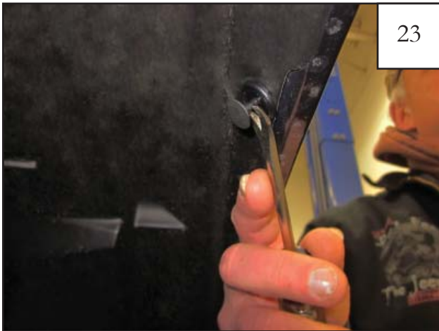
Using a pry tool, remove two plastic factory fasteners. Reference Step 22 for locations.
