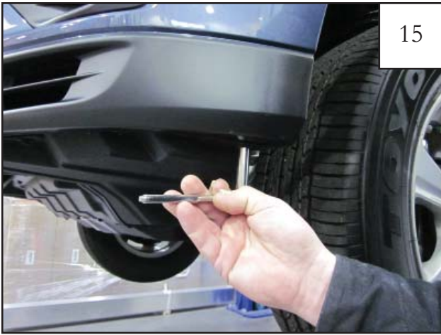
Using a 10mm socket wrench, remove factory bolt at front underside of wheel well. Save for reinstallation.
