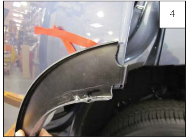
Open rear door and position Inner Door Piece on door. At top of part, align Inner Door Piece such that the breakaway tab hooks over the door lip.
