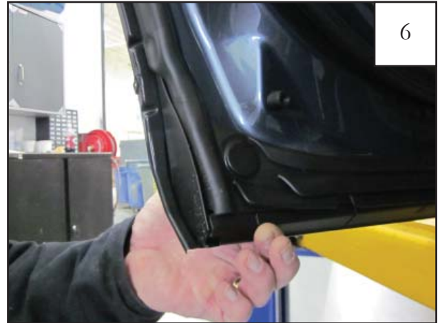
At bottom of part, align Inner Door Piece to nest snugly to lower curvature of the door.
