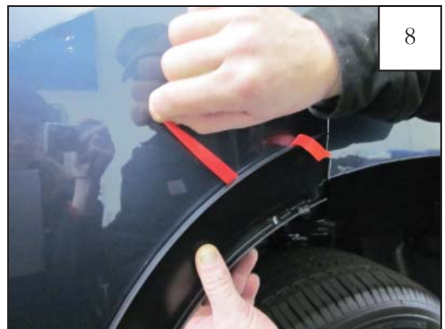
Pull red tape liner on the left (tape closest to edge of door).
