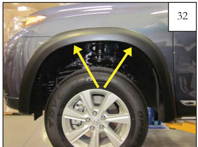
Hold flare to vehicle. Start Screws (SW1-0058) through two uppermost locations with #2 Phillips Screwdriver. Do not tighten.
