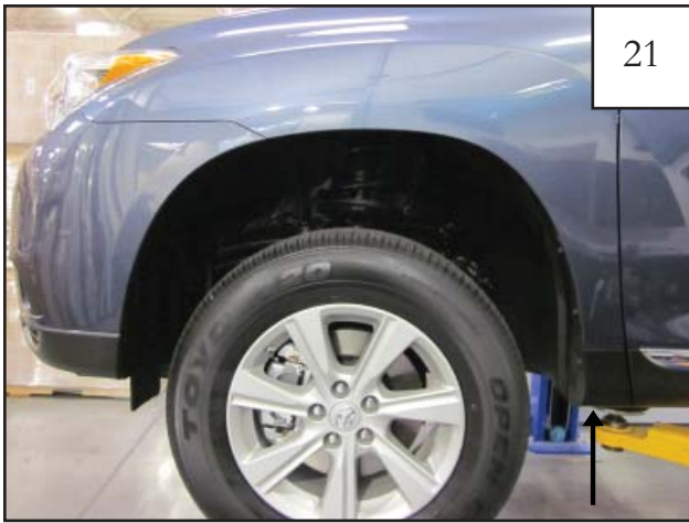
Using a pry tool, remove plastic factory fastener at lower rear of wheel well.
