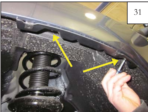
Hold front flare inner piece in wheel well with angled hole locations aligned with clips installed on wheel well lip in Step 26. Using a #2 Phillips Screwdriver, install Screws (SW1-0058) through front flare inner piece, through wheel well liner, and into Clip. Make sure that the corners of the Front Inner Piece are mounted flush with the sheet metal.
