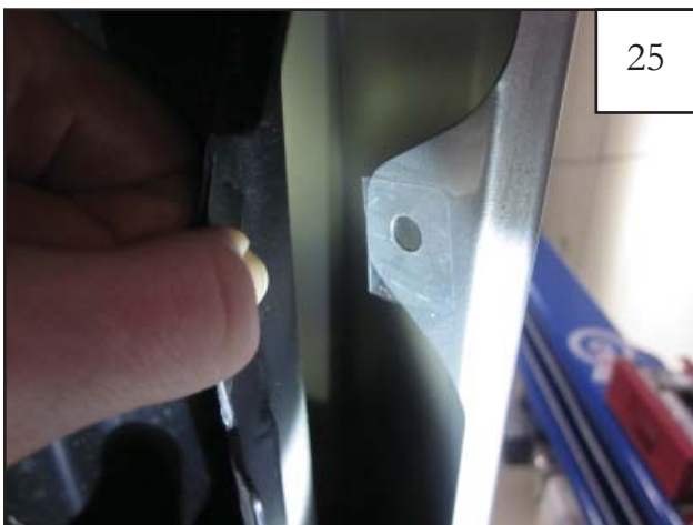
Install Tab (MT1-0014) over factory hole locations behind wheel well liner. Reference Step 22 for locations.
