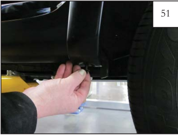
Install a Tuflock (RV1-P001) through hole drilled in previous Step.
