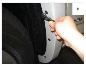
Start supplied truss-head screws through three rear holes in flare and into factory holes in rear of wheel well.
