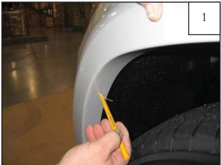
Hold the flare firmly on the fender. Using three forward holes in the flare as a guide, mark three clip locations with a grease pencil.
