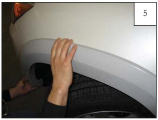
Replace flare on fender, aligning holes with the holes in clips.
