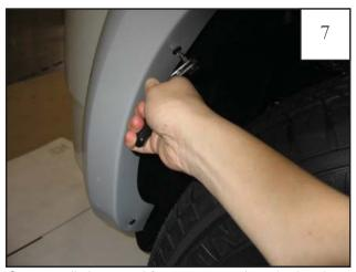
Start supplied serrated-flange screws through the three forward holes in flare and into the "S" clips installed in step 4. Using a right angle or stubby Phillips #2 screwdriver, tighten all screws.
