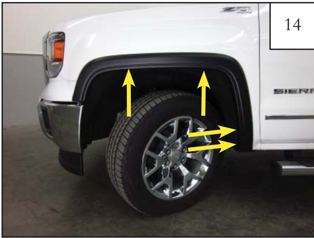
14 While holding Flare on vehicle, install supplied screw (SW1-0056) into the four factory hole locations as shown. Do not fully tighten at this time.
