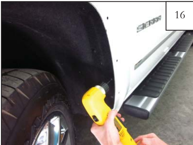
16 Remove the flare. Using a 3/32" drill bit, drill a pilot hole through the factory wheel well liner and sheet metal at location marked in previous step.
