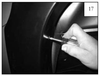
Start a supplied Screw (SW1-0050) through each of the remaining holes and into each Clip installed in Step 15. If needed, use scratch awl to locate holes.
