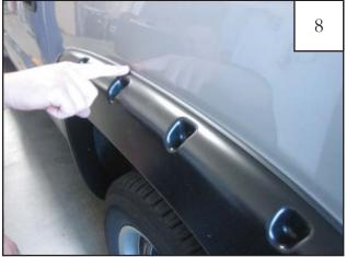
Ensure that the topmost edge of the flare is seated in the groove of the vehicle body.
