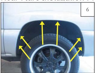
Place Clips (CL1-0022) over the six factory holes that line up with the holes in the fender flare. *NOTE:* There may be extra factory holes not used for installation.
