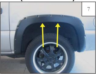
Hold rear flare in place on fender and start the top two Screws (SW1-0056), threading them through the flare, the Clips, and into the factory holes. *Do not tighten.*
