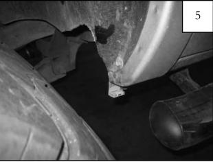
Install assembled Clip (CL1-0008 & CL1-0010) onto rear edge of front fender, aligning clip with edge of fender as shown. The snap lock feature of the Clip should be facing outward.
