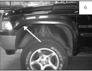
Position flare on fender, pushing flare tightly against fender. Using a right-angle drill with a #2 Phillips bit, drill one supplied Screw (SW1-0066) through plastic of fender flare and into sheet metal of fender using the indents in the flare as a guide.
