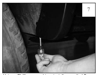
Using a Phillips screwdriver, install a supplied Screw (SW1-0049) into Clip (CL1-0008 & CL1-0010) installed in Step 5.
