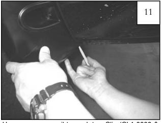
Use a grease pencil to mark two Clip (CL1-0008 & CL1-0010) locations using the two lower holes in the flare as a guide.
