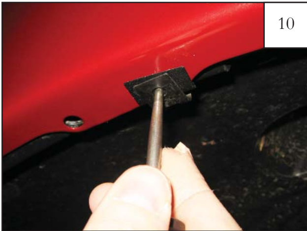
10 Using an awl or similar pointed tool, poke a hole through Tab (MT1-0014) using the Clip (CL1-0022) hole as a guide.
