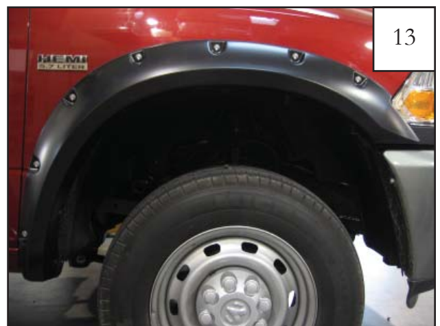
13 Completed front flare installation.
