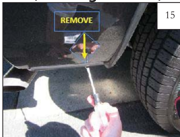
2012 - 2014 Models Only (Optional): Remove inner piece at bottom rear of wheel well using a pry tool.
