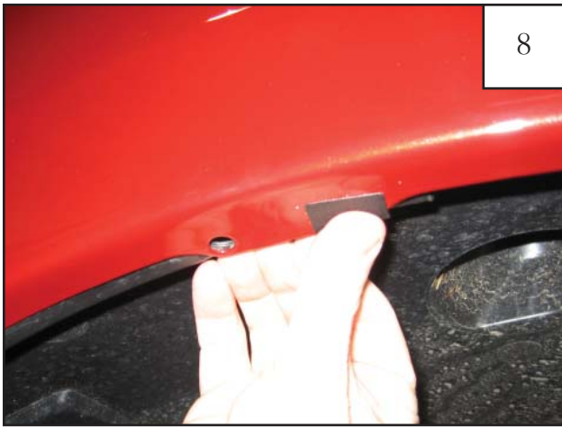
8 Install Tab (MT1-0014) over existing factory hole. There are two holes at the top center location. Refer to step 7 for proper hole for installation.
