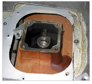
Clean up any residual silicone gasket material from the top of isolator and the transmission case.
