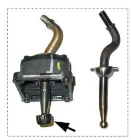
Using a number T-25 Torx bit, disassemble the shift tower.
