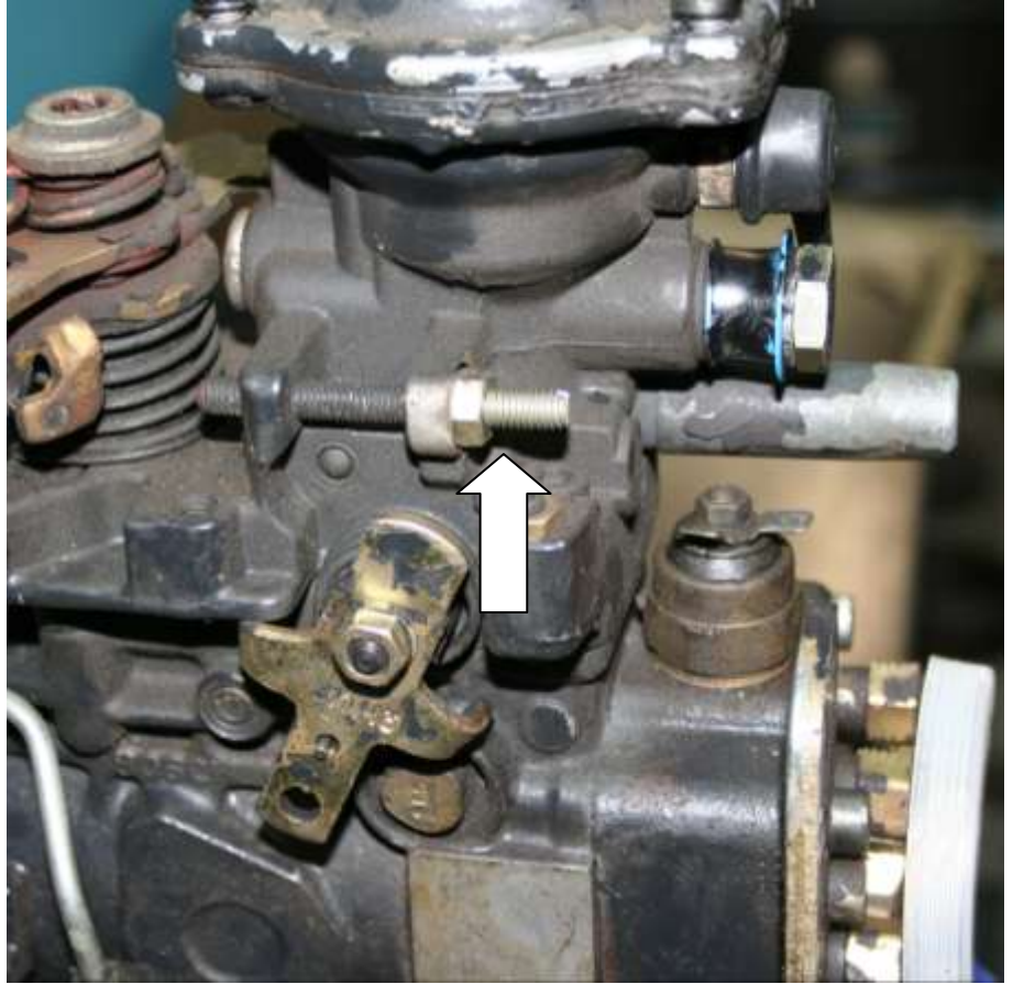
Picture shows cap and extra jam nut removed.
