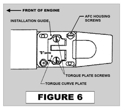
possible so that there is nearly zero clearance between the front of the torque plate and the installation guide.
