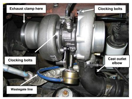
Connect the oil drain tube to the bottom of the turbo using the supplied gasket and the original hardware. You will need to slide the oil drain adapter as far as possible away from the wastegate arm to prevent any contact. In some rare cases the wastegate arm may need to be bent.
