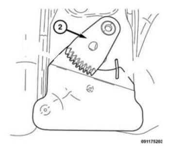
Align the hole on the sector gear to the hole in the CHRA towards the turbine side. Keep in place, do not allow movement.
