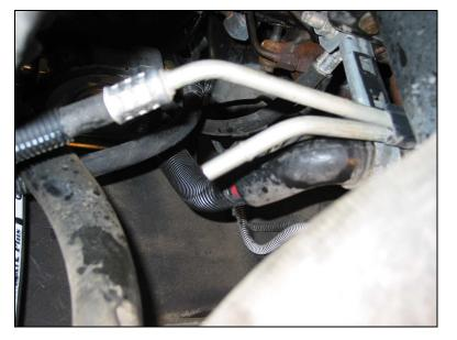
Push a hose clamp over the outlet hose from the filter and attach the hose to the straight fitting just installed on the steel line, cutting any excess hose. Tighten the hose clamp.
